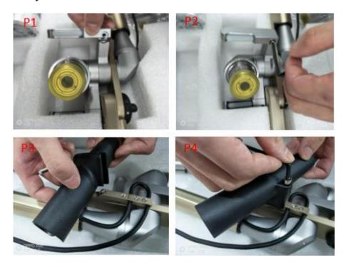
Step 2: Install the joints arm weight.
